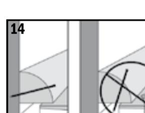
An expansion gap T-strip is required when length of planks measure 40' max and when width of planks measures 25' max. Transition strips must be placed in all doorways directly under the door when the door is closed.
