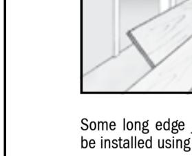
To measure and cut last piece in a row, rotate offcut section 180°, mark accordingly, cut, rotate back 180° and slot into space.
