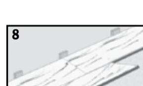
Remove the tongue on the panels that abut the walls to allow room for spacers and prevent problems from spills.
