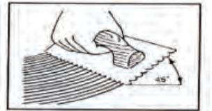
**Note:** Change the trowel every 2000 to 3000 square feet due to wear down of the notches. This assures you always get the proper spread of adhesive.
